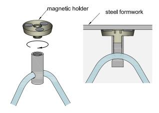
Protective Caps (for more information, look at brochure "Threaded Lifting System", page 6) are used to seal Concrete Anchor and prevent various substances such as residual concrete, dust, snow etc. from penetrating into the Concrete Anchor, protecting the anchor thread from clogging up.
