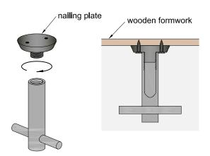
Magnetic Holder – Type HM4 (for more information, look at brochure "Threaded Lifting System", pages 2-4) are used when is necessary to fasten Concrete Anchors to a steel formwork
