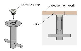
Lifting Eye, Treaded Lifting Loop, Threaded Lifting Loop with pressure plate and Lifting Loop "Goliath" (for more information, look at brochure "Threaded System Accessories" page 8-15) are to be used as lifting devices of the Thread System. They must be completely screwed into the Concrete Anchors.
